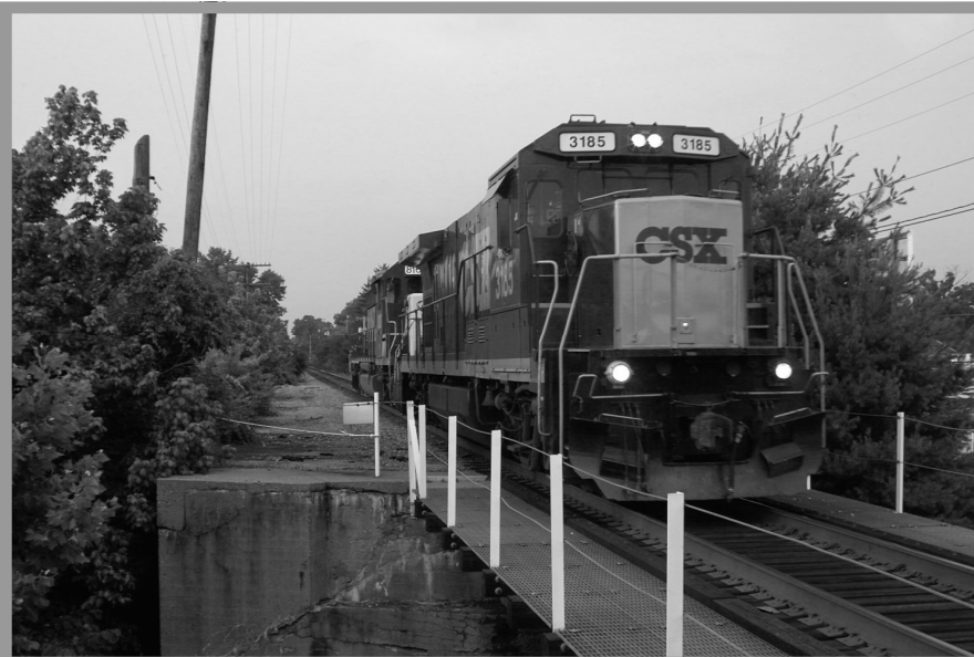
A CSX light engine move from Atkinson to the Ft Campbell interchange south of Hopkinsville. The lead unit, CSX 3185, is a unique engine - a GE B23-7R - with only 2 on the CSX roster. This unit was originally a Western Pacific B23-7 and still rides on its as-built EMD trucks. 6/27/05 Digital image by Chuck
